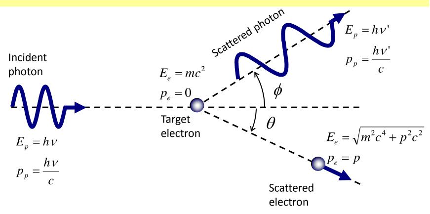
loss in photonenergy = gain in electron energy hv - hv' = KE
