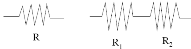
Figure 2: The schematic representation of a resistor (left) and two resistors in series (right).
